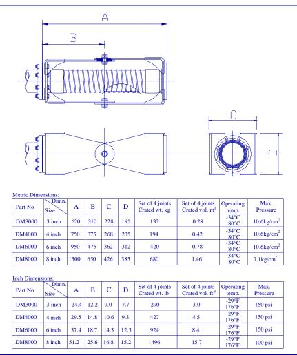
Materials: The standard BTE Drain Joint hose is constructed from layers of polypropylene and polyester film and fabric. Hoses have 316 stainless steel inner and outer wires and are swaged to carbon steel tailpieces with ANSI 150# RF flanges. Flanges can also be in stainless steel or in carbon steel, epoxy painted. The BTE Drain Joint pivot assembly is stainless steel with main side plates either standard galvanised or stainless steel.
